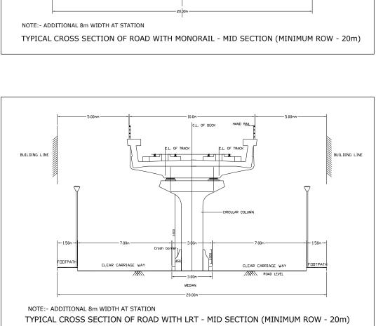
Figure 6.9 Typical Cross-Sections of Road with Elevated LRT and Monorail
