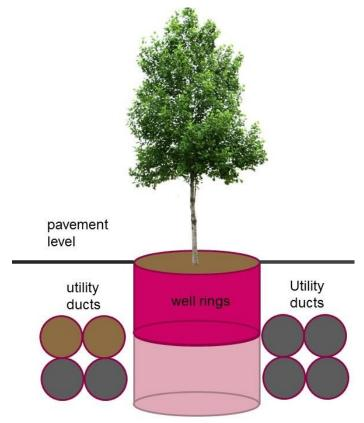
In the TenderSURE context, this can be easily done by using rings made of **ferrocement**. It is economical also.
